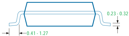
Recommended Solder Pad Layout
